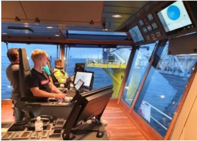
FIGURE 30 - TYPICAL DP STATION WITH VIEW OF THE GANGWAY
