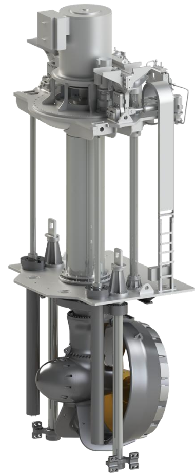
FIGURE 47 - TYPICAL RETRACTABLE AZIMUTH THRUSTER (1)
