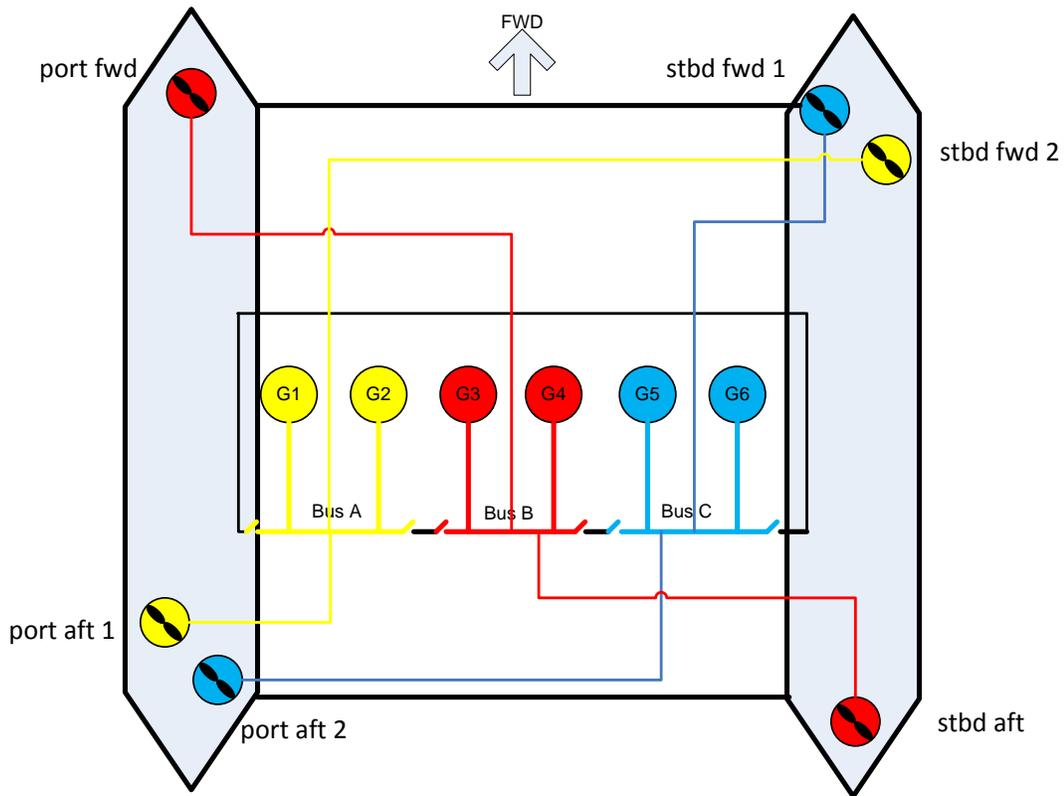
Figure 1 Simple schematic layout of Propulsion Power System
